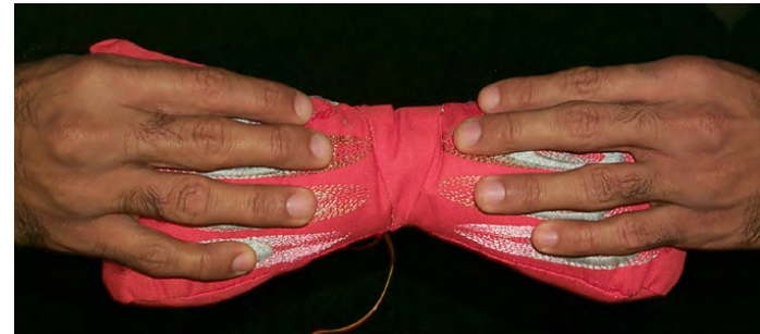
Figure 12.14 Melody Butterfly designed for piano-like finger-by-finger control.
